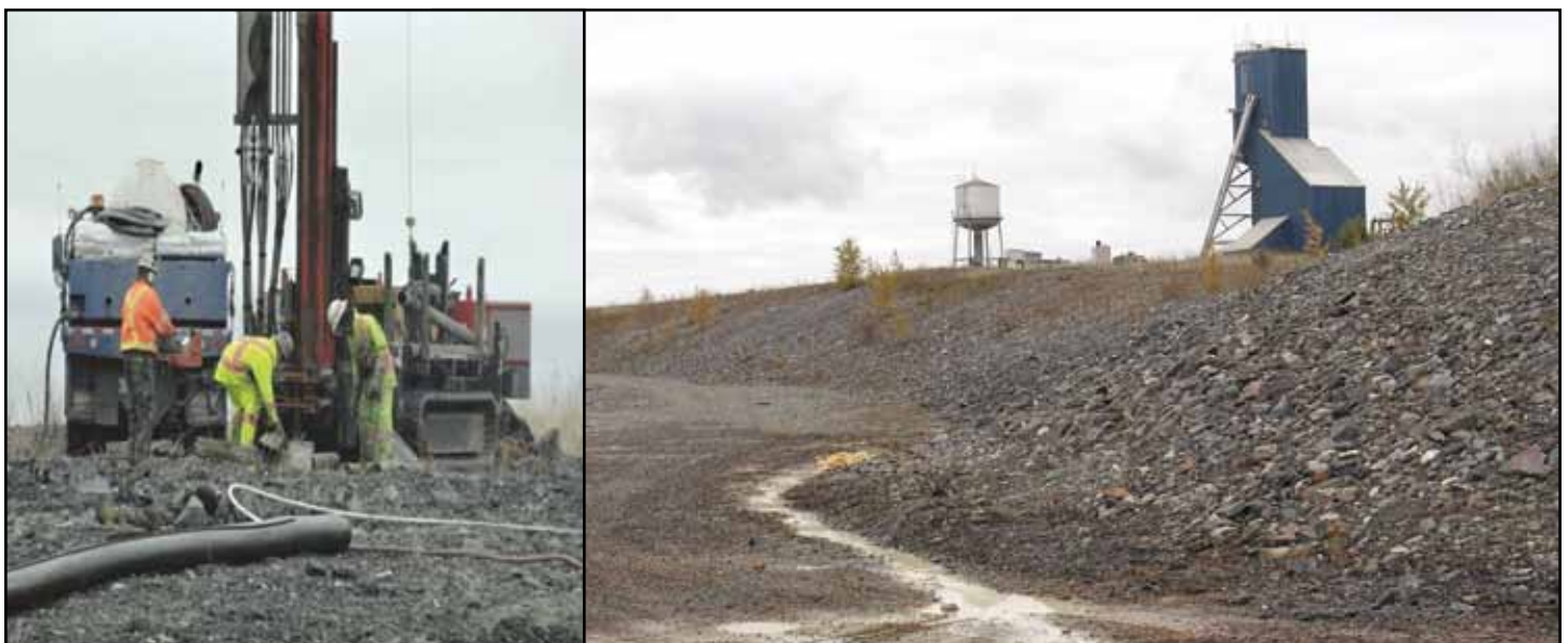
BacTech drills to test mineralization in concentrate stockpiled for over 50 years in Snow Lake, Manitoba prior to investigating feasibility of applying its proprietary bioleaching technology to clean up the toxic site and reclaim up to $150 million in gold contained in the ore.
